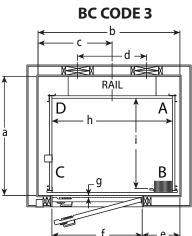
\*All dimensions are finished hoistway dimensions **CB CODE 3**
